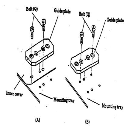
Figure 1-13. Guide Plate Installation
